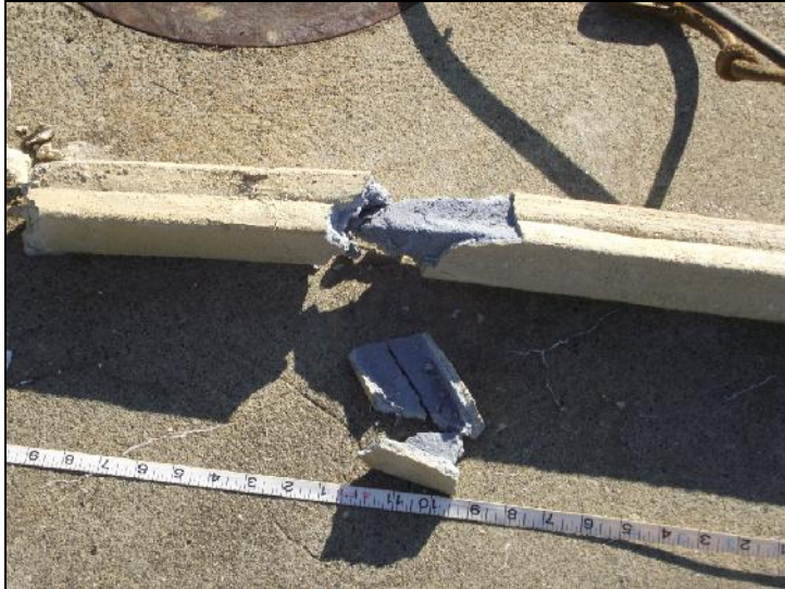
Close-up of anode, shows deterioration of zinc
